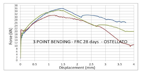
Fig. 4: Test result of FRC notched beams
