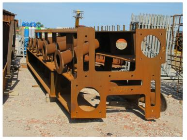
Fig. 3: The stay anchorage frame (2 each towers)
